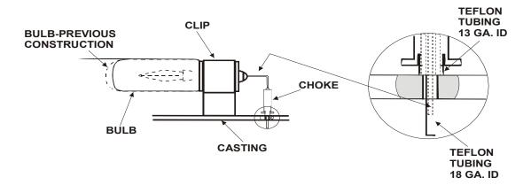
Figure 58. Ignitor Bulb
